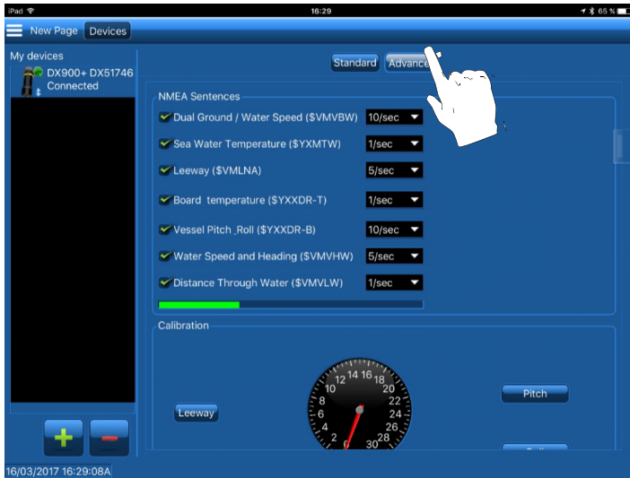
Figure 19. Enabling/disabling NMEA sentences and changing the refresh rate (Speed & Temperature sensors only)
